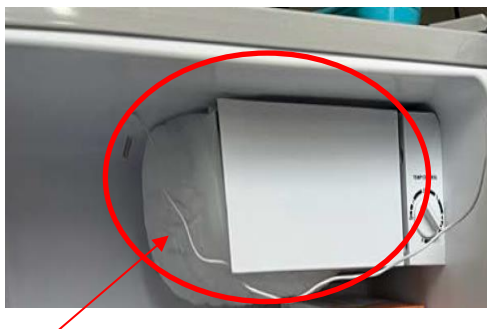
Figure 3. Frost may form inside the freezer compartment
